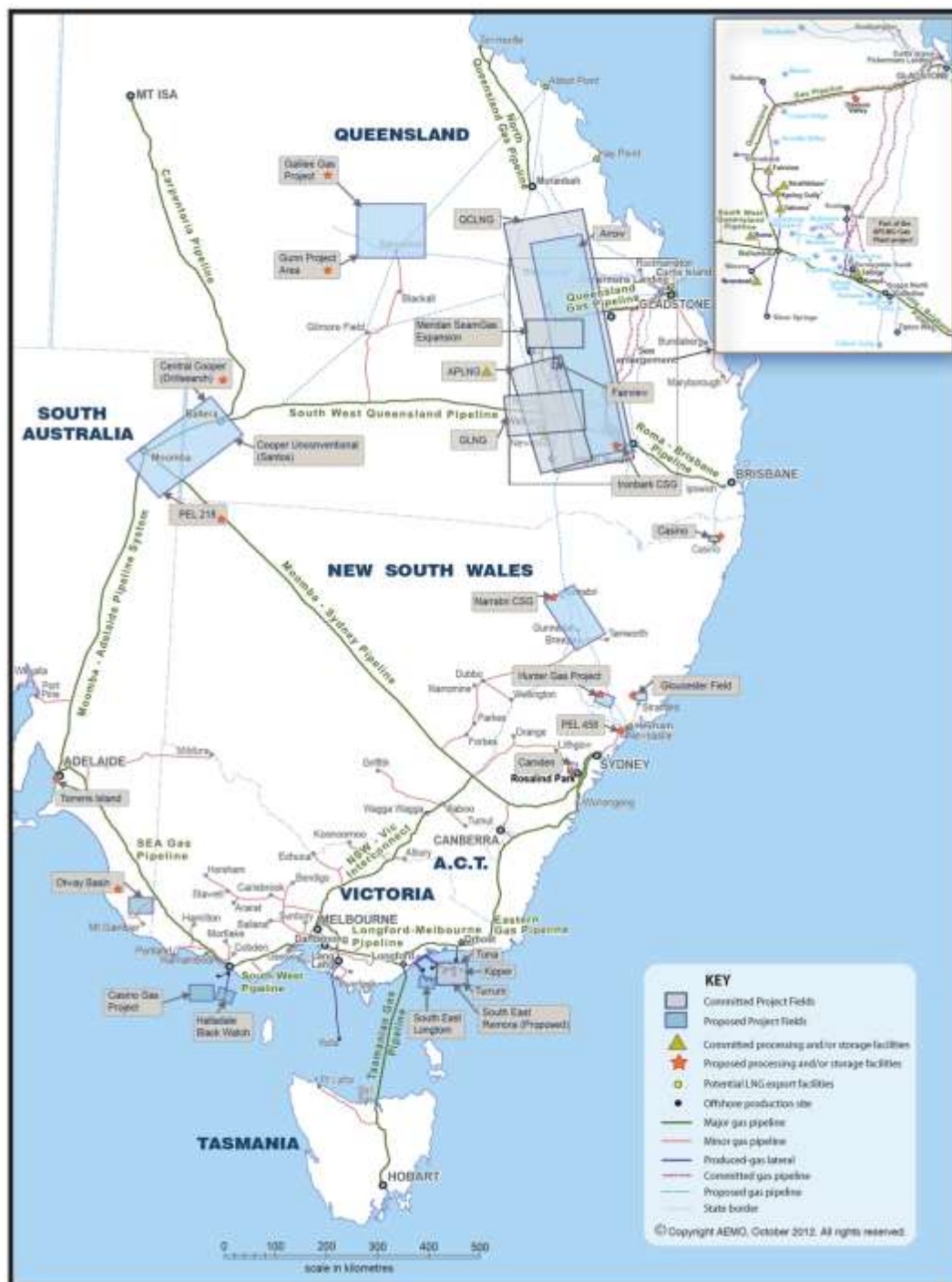
Figure 1: Eastern Australian committed and proposed gas supply facilities and transmission pipeline systems (2012 AEMO GSO)
